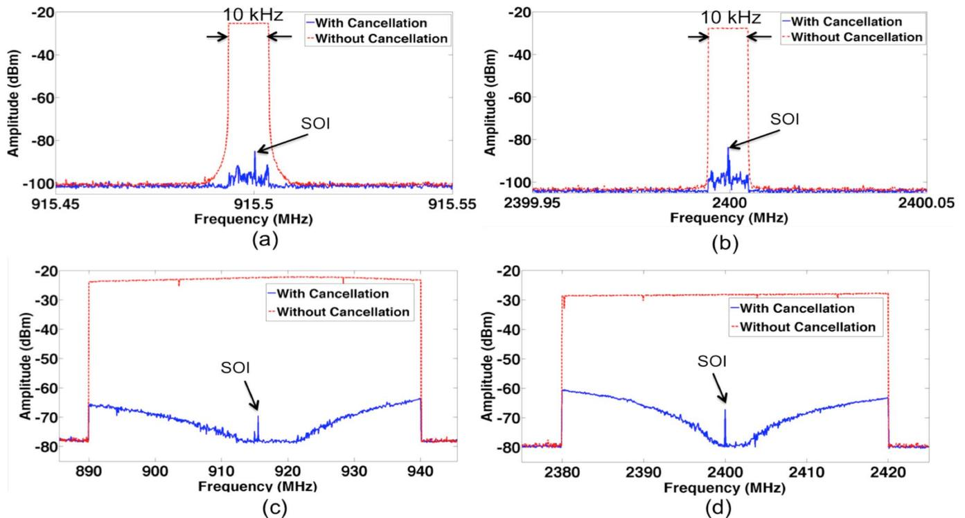
Fig. 2. Spectrum of the received signal before (dotted line) and after (solid line) applying the EAM interference cancellation system for a (a) 900 MHz narrowband interferer, (b) 2.4 GHz narrowband interferer, (c) 900 MHz broadband interferer, and (d) 2.4 GHz broadband interferer. SOI = signal of interest.
