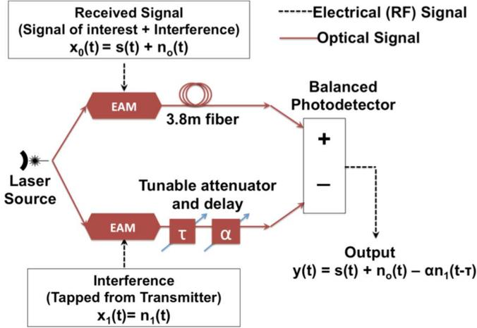
Fig. 1. Schematic of the EAM interference cancellation system.
