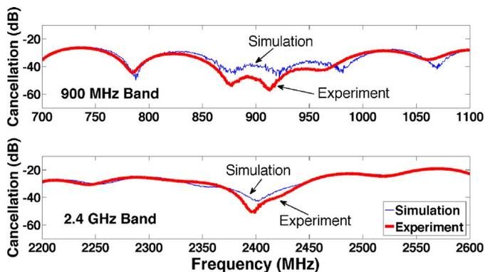
Fig. 3. Cancellation profile across 400 MHz bandwidth in both the 900 MHz and 2.4 GHz bands. Experimental results are given by the thick, red line while simulation is given by the thinner blue line.
