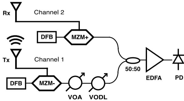
**Fig. 1** Optical cancellation system architecture. Channel 1 carries the interference signal to the negative quadrature biased modulator, variable optical attenuator, and variable optical delay line. Channel 2 refers to the receive antenna output, which is coupled to the positive quadrature biased modulator. The two channels are then combined in a 50:50 optical coupler and amplified prior to the photodetector.
