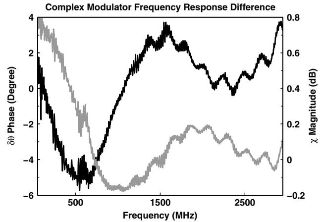
**Fig. 3** Measured difference in complex frequency response for the transmit and receive channel modulators. (Black) represents phase mismatch  $\delta\theta$ , labeled on the y-axis left in degrees. (Gray) represents magnitude mismatch  $\chi$ , labeled on the y-axis right in dB.
