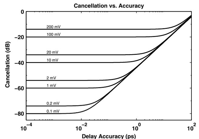
**Fig. 2** Calculated cancellation of a 1 GHz signal with varying attenuation and delay device accuracy according to Eq. (10). The values for attenuation accuracy  $\Delta\gamma$  are labeled with their associated plots and correspond to values ranging from 0.1 to 200 mV.
