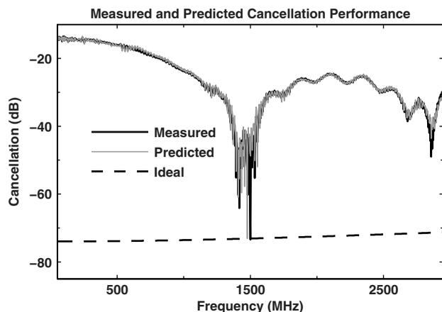
**Fig. 4** Measured broadband cancellation compared with simulated cancellation performance, with values for attenuation and delay precision of  $\Delta\gamma = 0.2$  mV and  $\Delta\tau = 0.01$  ps. Predicted cancellation is based on Eq. (11) and incorporates the measured difference in complex modulator frequency response to produce values for  $\chi$  and  $\delta\theta$ . Ideal cancellation corresponds to precision limited performance where  $\chi = 0$  dB and  $\delta\theta = 0$ .
