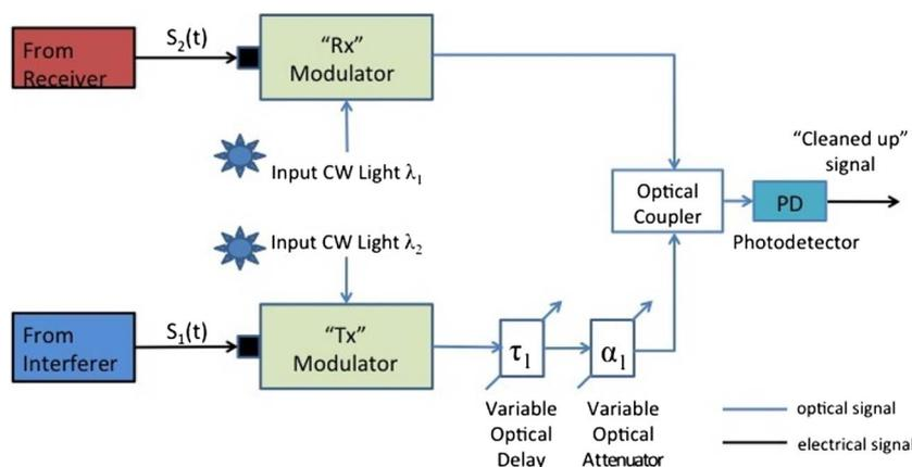
Fig. 1. System architecture for the incoherent OCS. Rx = received signal arm; Tx = reference/transmitted signal arm.
