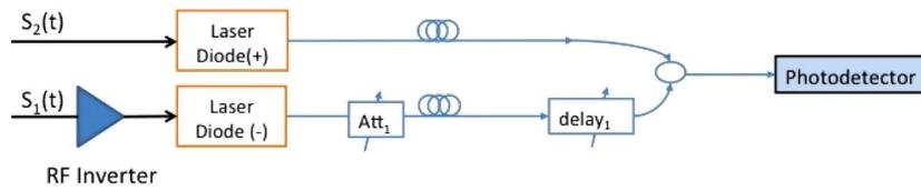
Fig. 3. System architecture for the direct modulation OCS.
