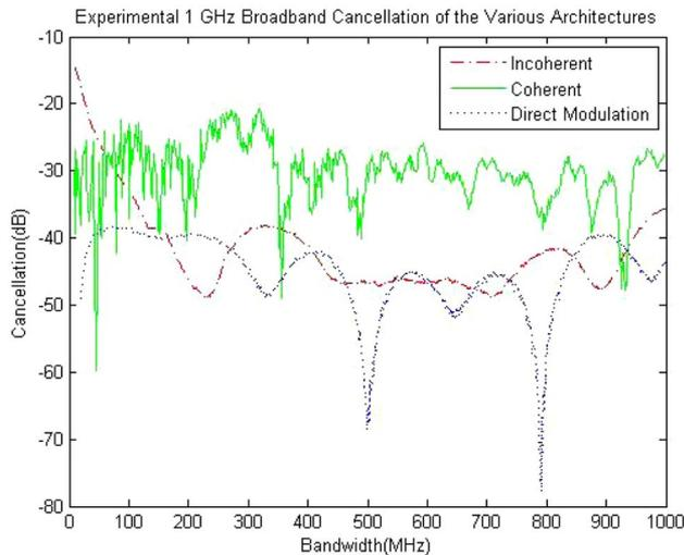
Fig. 5. Experimental depth of cancellation performance for broadband (1 GHz) cancellation for the incoherent, coherent, and direct modulation optical interference cancellation architectures.
