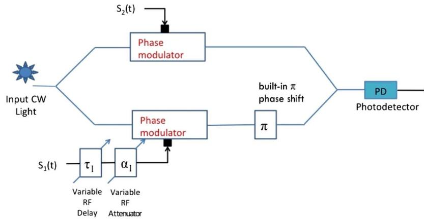
Fig. 2. System architecture for the coherent OCS.
