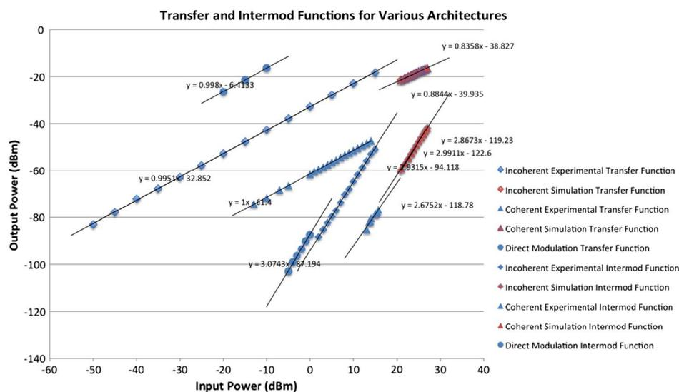
Fig. 4. Transfer functions and intermodulation functions for the incoherent, coherent, and direct modulation architectures. The linear-fitted trendlines indicate that the transfer functions have a slope of ~1 and that the intermodulation functions have a slope of ~3.
