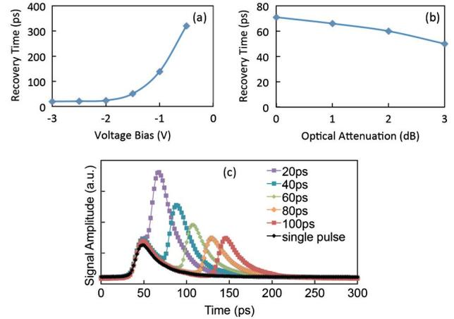
Fig. 2. (Color online) (a) Measured absorption recovery time as a function of EAM bias voltage. (b) Measured absorption recovery time as a function of optical pump-pulse attenuation. (c) Integration response of the EAM with different temporal separation of the pump pulses.
