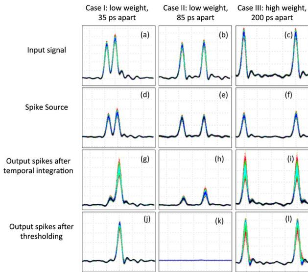
Fig. 4. (Color online) Experimental results of input, spike source, and output pulses in three different cases with different time intervals and weight values.
