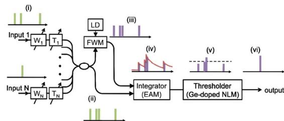
Fig. 1. (Color online) Illustration of an asynchronous spiking photonic neuron.  $W_1-W_N$ , variable weight;  $T_1-T_N$ , variable time delay; FWM, four-wave mixing; LD, laser diode; EAM, electro-absorption modulator; Ge-doped NLM, optical thresholder.
