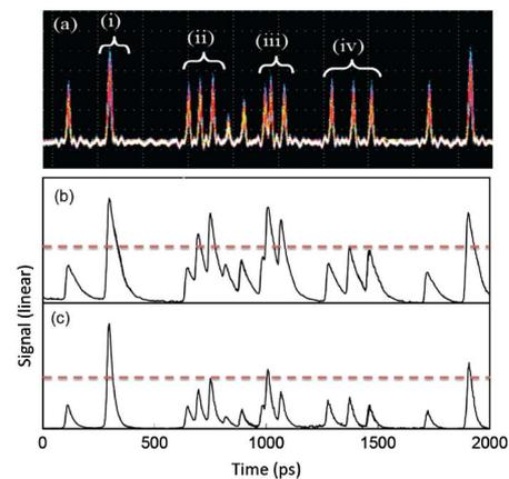
Fig. 3. (Color online) Time-sensitive signal integration in EAM: (a) input signal, (b) integrated output with long integration window, and (c) integrated output with short integration window.
