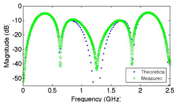
Fig. 2. Measured and predicted magnitude response of eight-tap FIR filter weighted  $[1.0914 \ 1.0617 \ -1.0715 \ -1.0814 \ -1 \ -0.9683 \ 0.9795 \ 0.9594]$ .
