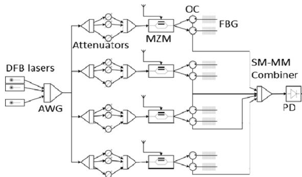
Fig. 1. Architecture for our photonic beamformer. DFB: distributed feedback laser, AWG: arrayed-waveguide grating, MZM: Mach-Zehnder modulator, OC: optical circulator, FBG: fiber-Bragg grating, PD: photodiode.
