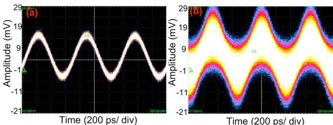
Fig. 3. Signal combination with a. SM-MM combiner b. SM-SM Coupler.
